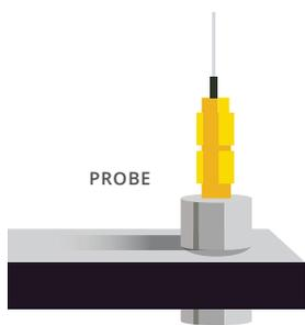
**Dielectric thickness measurements work best with materials that have good control over their dielectric content.**
