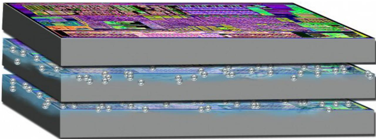
*Coplanarity ensures all connections are successfully bonded, minimizing the risk of field failure.*
