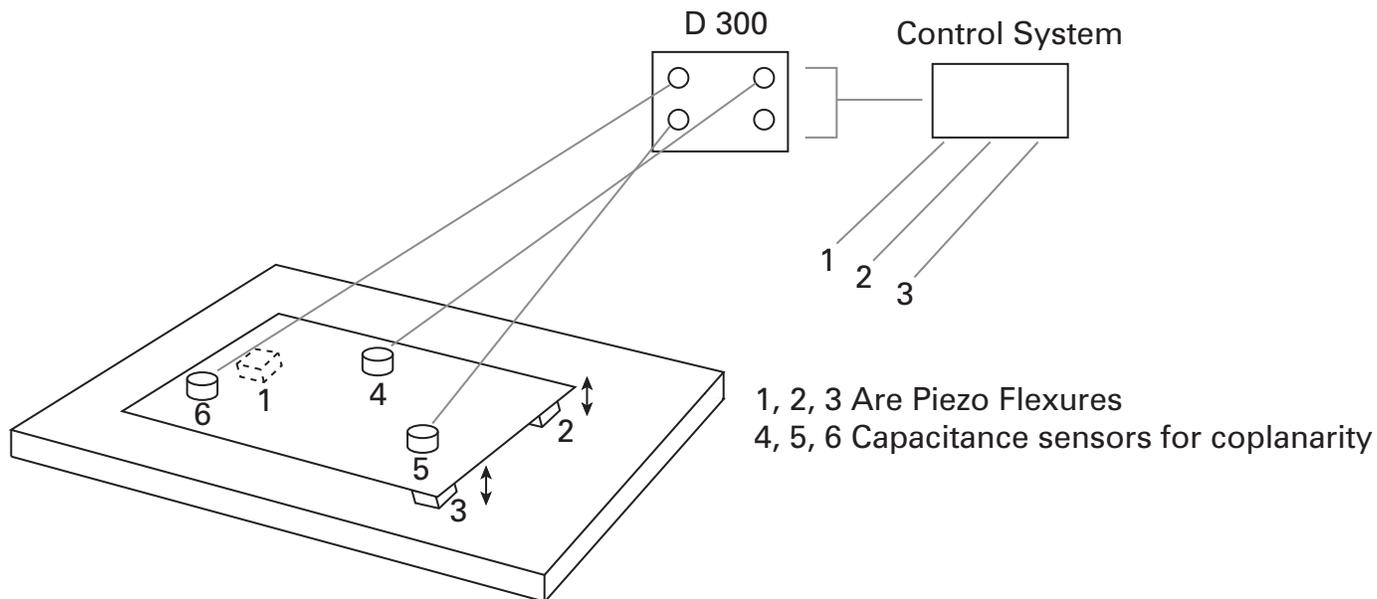
*Three gap measuring probes mount to the upper plane (die bonding tool). A control system monitors coplanarity of the tool to the lower plane (die or substrate) and provides position control to the actuators.*
